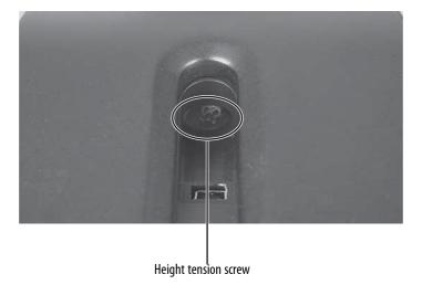
3 Adjust the height tension screw so the monitor stays in place when you let go. If the monitor lowers by itself when you let go, turn the screw clockwise several complete turns. If the monitor rises when you let go, turn the screw counter-clockwise several complete turns. You may need to turn the screw several times before the tension is correct for your size of monitor.
